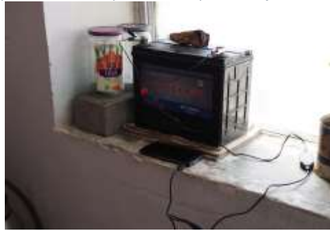
Figure 19 Using the old solar panel and battery as a back-up source of electricity. A mobile phone is charging.
